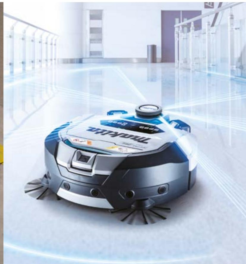
**LIDAR SENSOR + KAMERA SENSOR**
